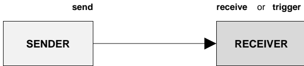
Figure 12. Illustration of message-based communication
